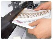
Pre-punched products are manually hung horizontally. A foot switch then activates the transportation and binding station, and the next wire is presented for the next product.
