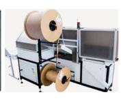
Spool de-winding with integrated paper separation re-winding
